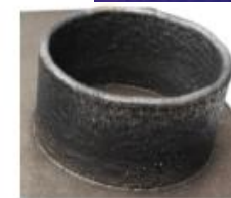
Part realized without CLAMIR: H = 25.00 mm W = 2.50 mm
