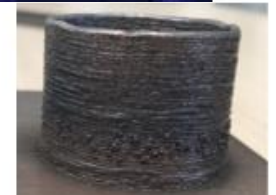
Part realized with CLAMIR: H = 26.00 mm W = 2.10 mm
