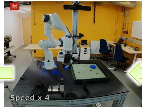
Generation and execution of a collision free trajectory to reach the assembly configuration
